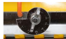
Uniform scatter, accurate spread width, adjustable agitator vanes
