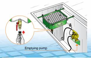
The drained oil can be transferred from the collection bowl to the storage tank by gravity or by using an emptying pump connected to the fixed system
