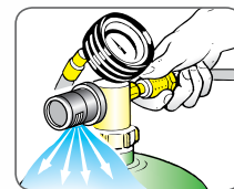
The air pressure for correct depressurisation is between 6,5 and 7 bar
