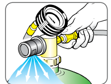
The air pressure for correct depressurisation is between 6,5 and 7 bar
