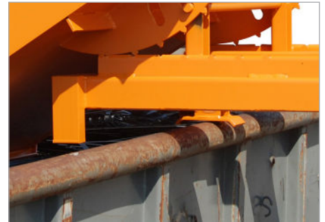
② manual release using the pull cable
